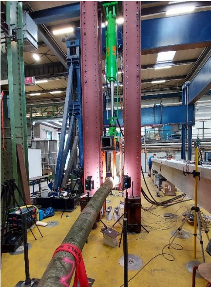
Bending test on the freshly cut shaft of a copper beech with the new long-stroke cylinder
