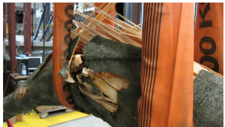
Bending test on the freshly cut shaft of a copper beech at the Institute for Building Research
